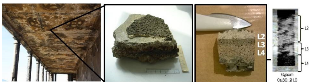
Figure 1. (A) A detail of the ceiling from the Punta Begoña inner areas where the concrete sample (B) was taken, (C) A cross section of the three mortar layers (L2, L3 and L4) over the concrete and the black crust formed over mortar layer L2, (D) Distribution of gypsum throughout the cross section of the three mortar layers over the concrete obtained using Raman imaging.
